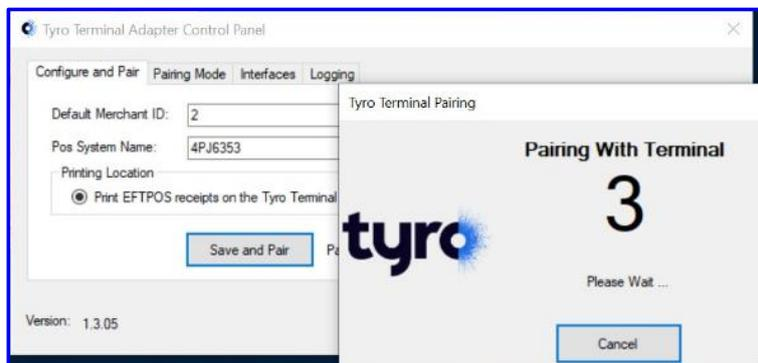
A window should appear with numbers counting up. When you see that press '**Start**' on the Tyro EFTPOS machine.
