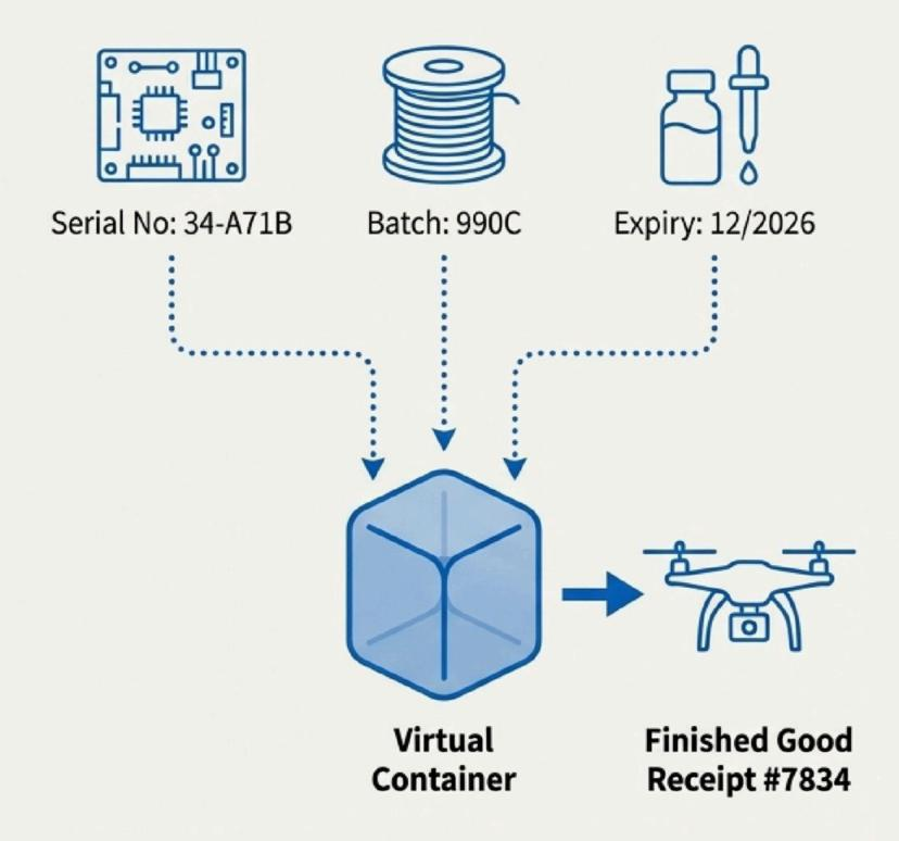
**Virtual Containers** link specific tracked components to a specific finished good receipt. This allows for pinpoint traceability of which components went into which finished product.
